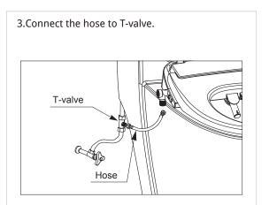
2. Existing water pipe connect T-valve.
