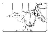
The product has no Ground Fault Circuit Interrupter, It should be installed in the line with Ground Fault Circuit Interrupter, Otherwise, the accidental failure of this product may result in the loss of life or property.
